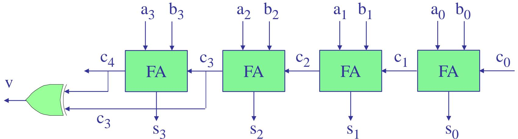
$$c_1 = g_0 + p_0 \cdot c_0 \quad (g_0 = a_0 \cdot b_0, \quad p_0 = a_0 + b_0)$$
