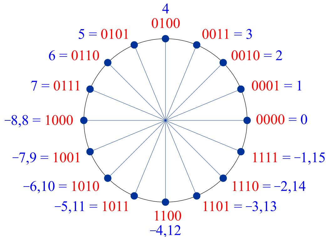
$$x = -b_3 2^3 + b_2 2^2 + b_1 2^1 + b_0$$
